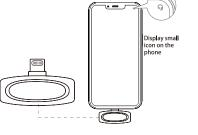
Step 2: Press switch key of microphone, the indicator light turns green, and then power is turned on.
