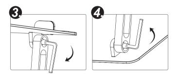
If the friction of hinge is too strong or too little for adjustment, you can use the wrench to adjust.
