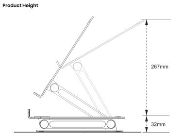
Above figure shows the reconmmended use range, but the stand is not fully extended in the figure.
